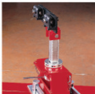
Column with anchoring clamp.
