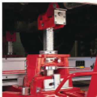
Vice. Accepts bushing or ridged heads. Lifting of the column by means of a ratchet.
