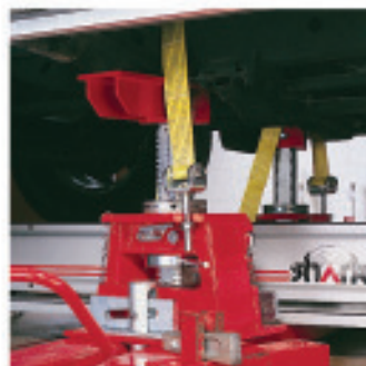
Wide support, squared, with strap and tensioner.
